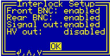
Fig. 5. Setting the interlock function in the dialog box "Interlock Setup".
