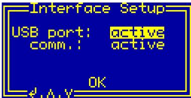
Fig. 7. Enabling the USB interface in the dialog box "Interface Setup".
