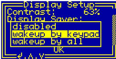
Fig. 11. Setting the display saver in the dialog box "Display Setup".
