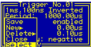
Fig. 28. Menu in the dialog box "Trigger" for selecting trigger settings.
